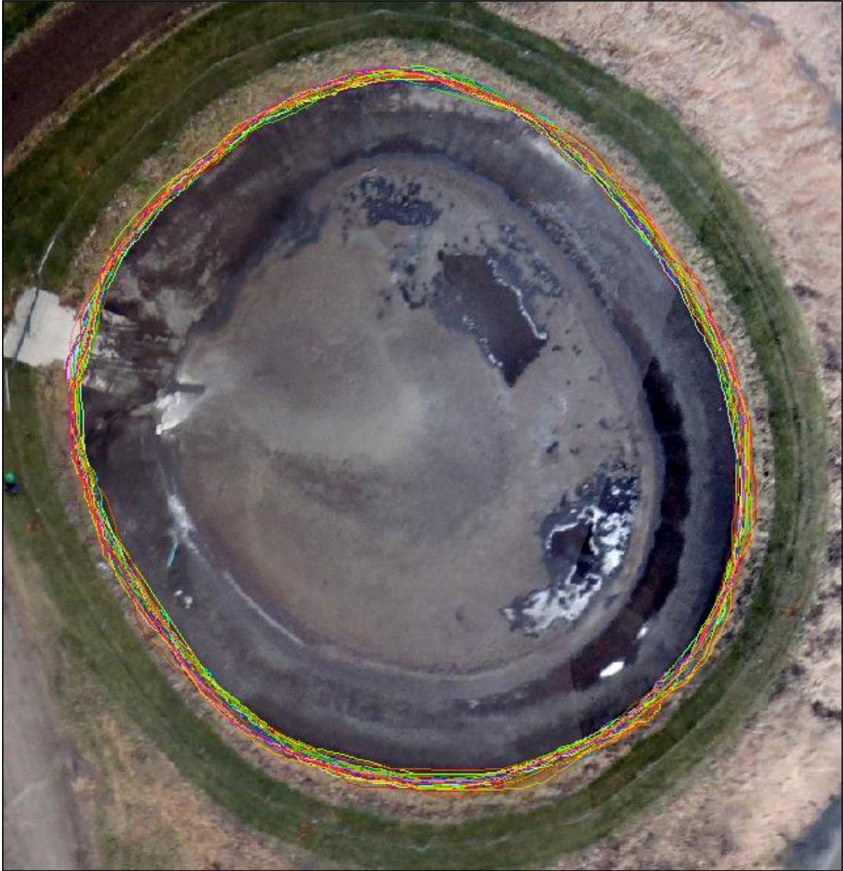
Figure 18: Superposition of 30 unique manure pit base polygons (sUAS)
