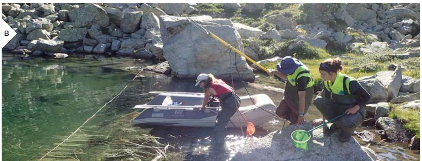
▲ **Figure 4.** Electrofishing in the lakes: A, use of heavy equipment; B, use of portable equipment with the operational help of a vessel and in combination with the strategic placement of shore nets.
