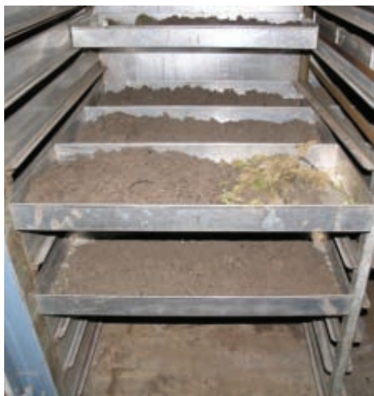
Contaminated soil drying on trays in an industrial dehydrator at 80 °C for 24 h. Photo: Elissa van Oosterhout
