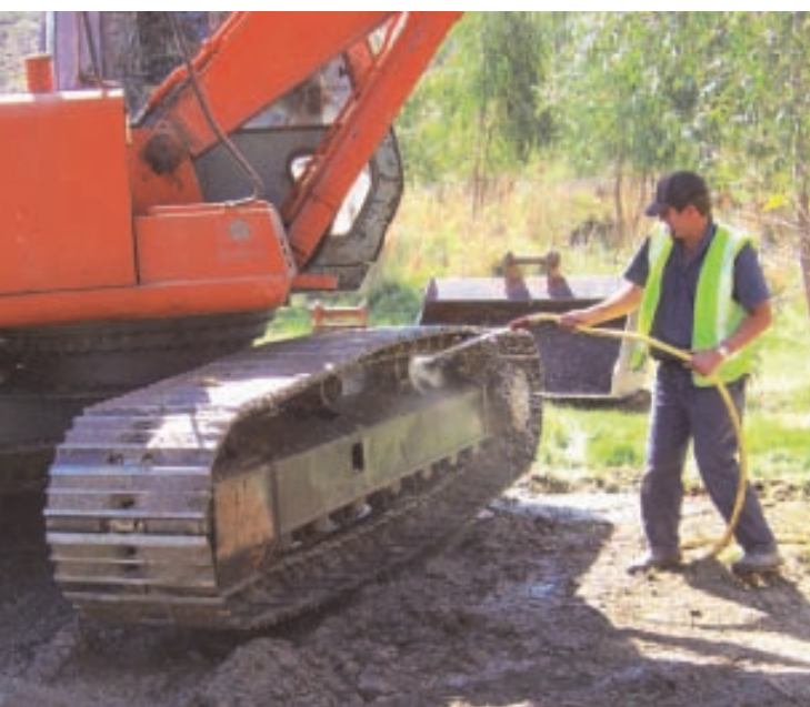
Machinery must be washed down. Photo: Thomas White
