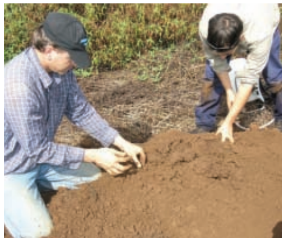
Soil must be hand-sieved until no more root fragments are found. Photo: Elissa van Oosterhout
