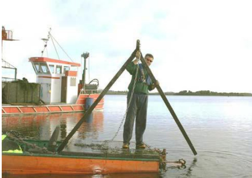
Figure 8.2: V-blade used to cut Curly Waterweed ( Lagarosiphon major ) in Rinerron Bay, Ireland (Caffrey & Acavedo, 2007; Photo reproduced with permission of J. Caffrey, Inland Fisheries Ireland).
