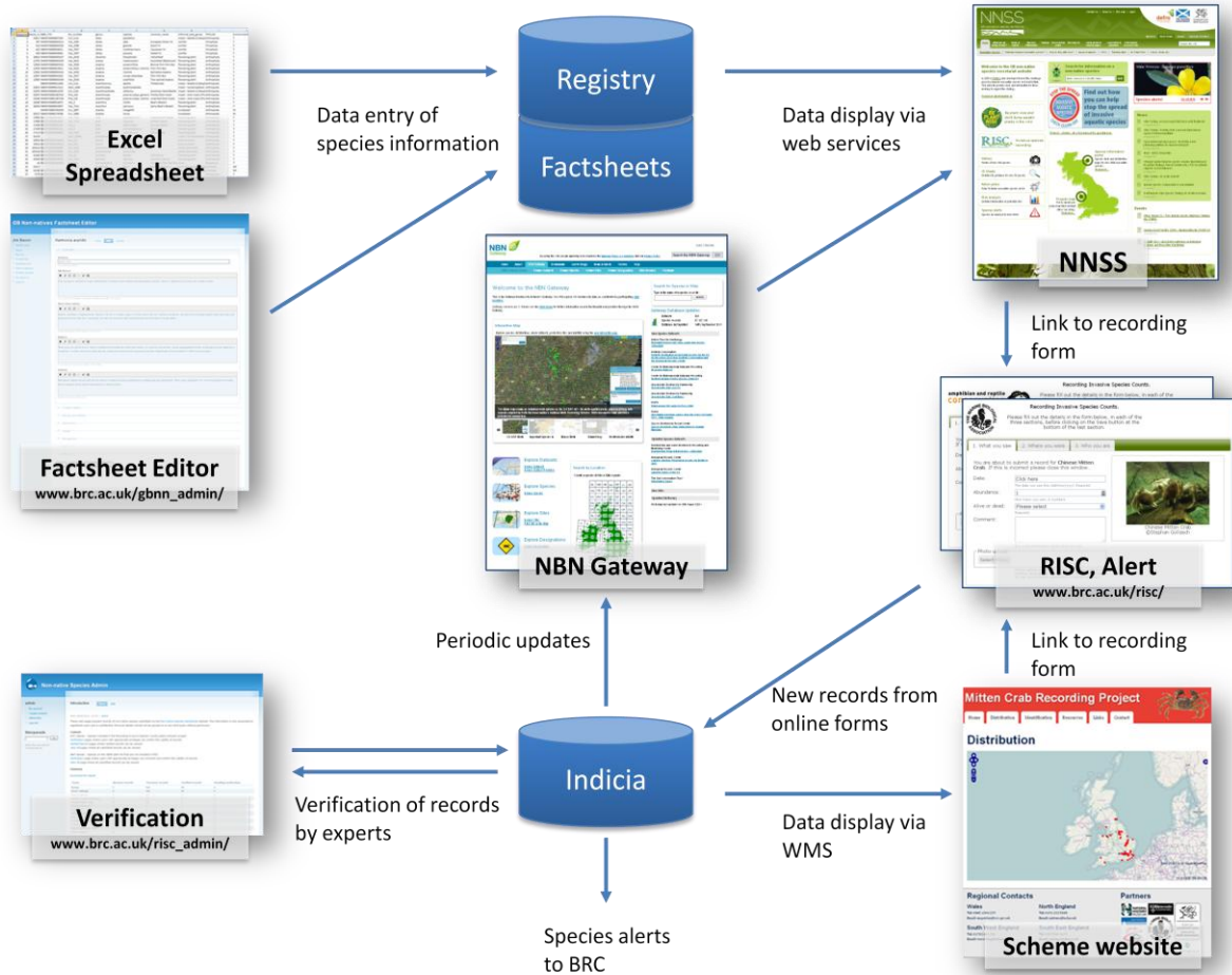
Figure 1b. Structure of the GB-NNSIP illustrating links between databases and web services which provide information to the GB-NNSIP within the Non-Native Species Secretariat (NNS) website.
