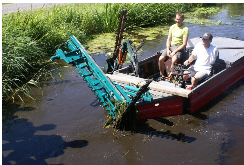
Figure 3.5: A weed cutting boat with adjustable mowing gear used for aquatic weed control in the Netherlands (Photo: R. Pot).
