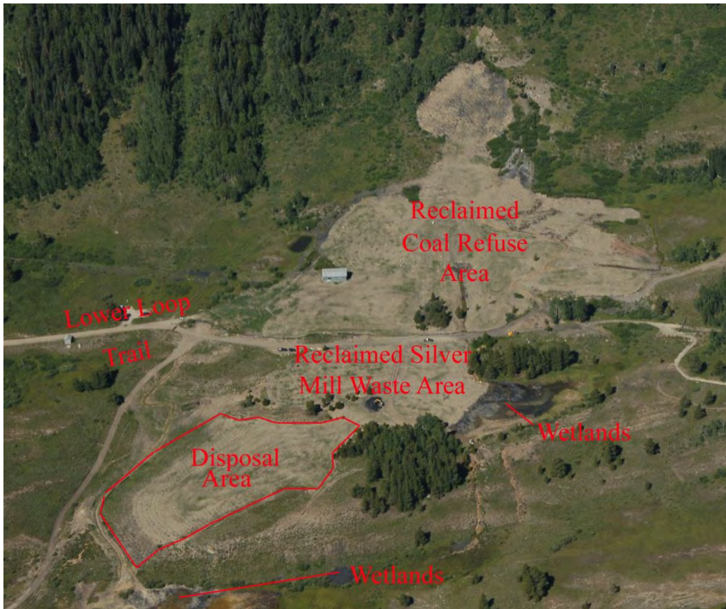
Figure 3. Aerial View of Peanut Mine, Early Summer Following Completion of Reclamation Construction.
