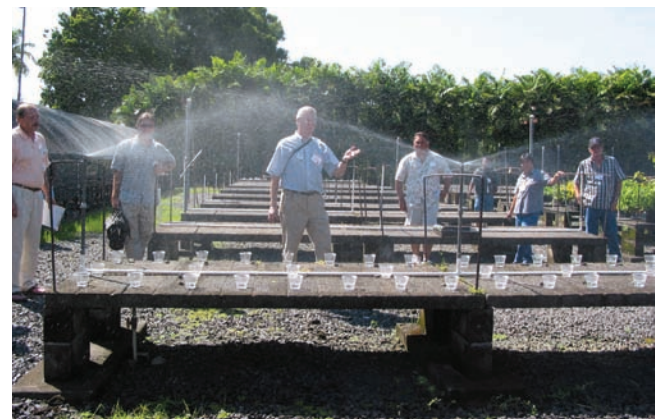
Figure 10.21 —Periodic checks of water distribution can easily be done with a “cup test” in which cups are arranged in a grid pattern. The depth of water in them is measured after a standard watering period. Photo by Kim M. Wilkinson.
