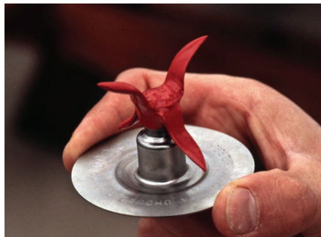
Figure 7.15 —Modifying kitchen blender blades by using rubber coating allows the grower to clean small lots of dry and fleshy fruits without damaging the seeds. Photo by R. Kasten Dumroese.
