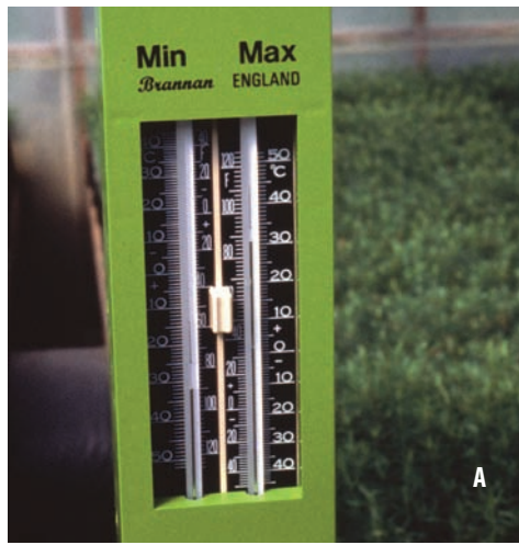
Figure 4.17 —(A) Monitoring and controlling temperature is critical to successfully growing a crop of native plants, and monitoring equipment is inexpensive. Many nurseries use thermometers that record daily maximum and minimum temperatures and (B and C) small, programmable, self-contained temperature sensors. Photo A by Thomas D. Landis, B and C by David Steinfield.
