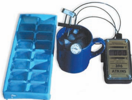
Figure 13.12 —(A) Temperature can be monitored with long-stemmed electronic thermometers. (B) Small devices such as the iButton® can monitor temperature for weeks or months and the data can be downloaded to a computer. (C) Calibrate any thermometer in a water-ice mixture to make sure it is accurate. Photos A and C by Thomas D. Landis, B by David Steinfeld.
