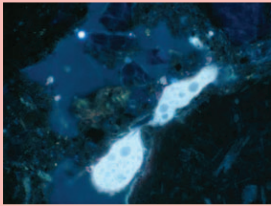
Figure 5 We have developed the biological thin-section technique, and used it to study the spatial distribution of micro-organisms and pore-space in soil. This has been used to develop 3-dimensional models of organism distribution in relation to water and solute (including pesticide) transport
